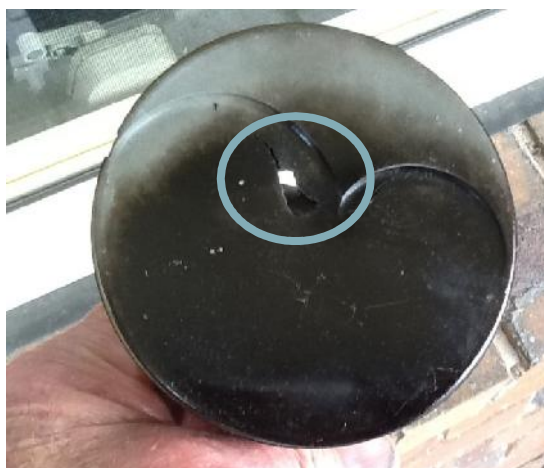
Right: Even a high end forged piston has no chance against extreme pressure and high temperature. What more intriguing, it the piece went out the exhaust without a mark on the seat.
