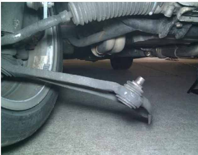
Above: A failure like a ball joint breaking off could be highly dangerous
