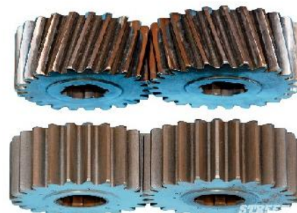
Above: Helical versus Spur gears Left: Spur gear geometry
